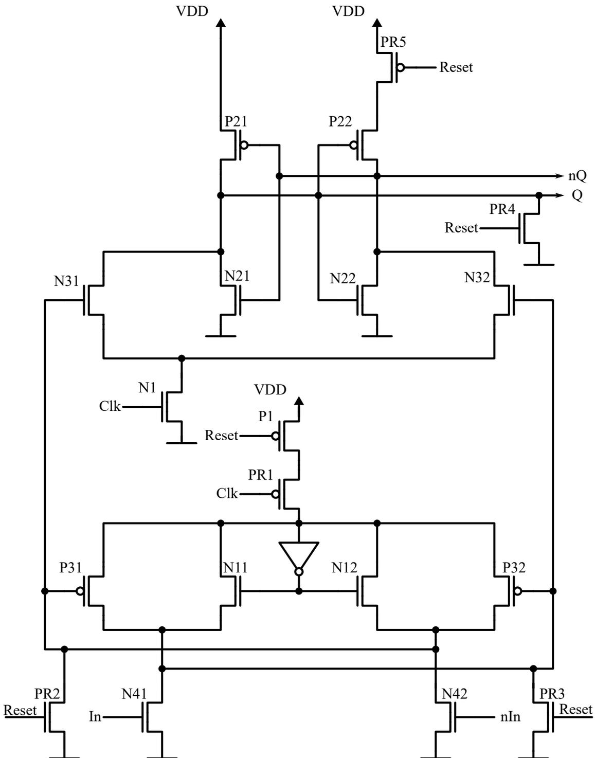
Figure 4.9: Implementation of the fully differential master slave D-flipflop with reset functionality. Notice that all MOSFETS shown are enhancement type FET's, bulks of NMOS transistors are always connected to  $GND$  and bulks of PMOS transistors are always connected to  $V_{dd}$ .
