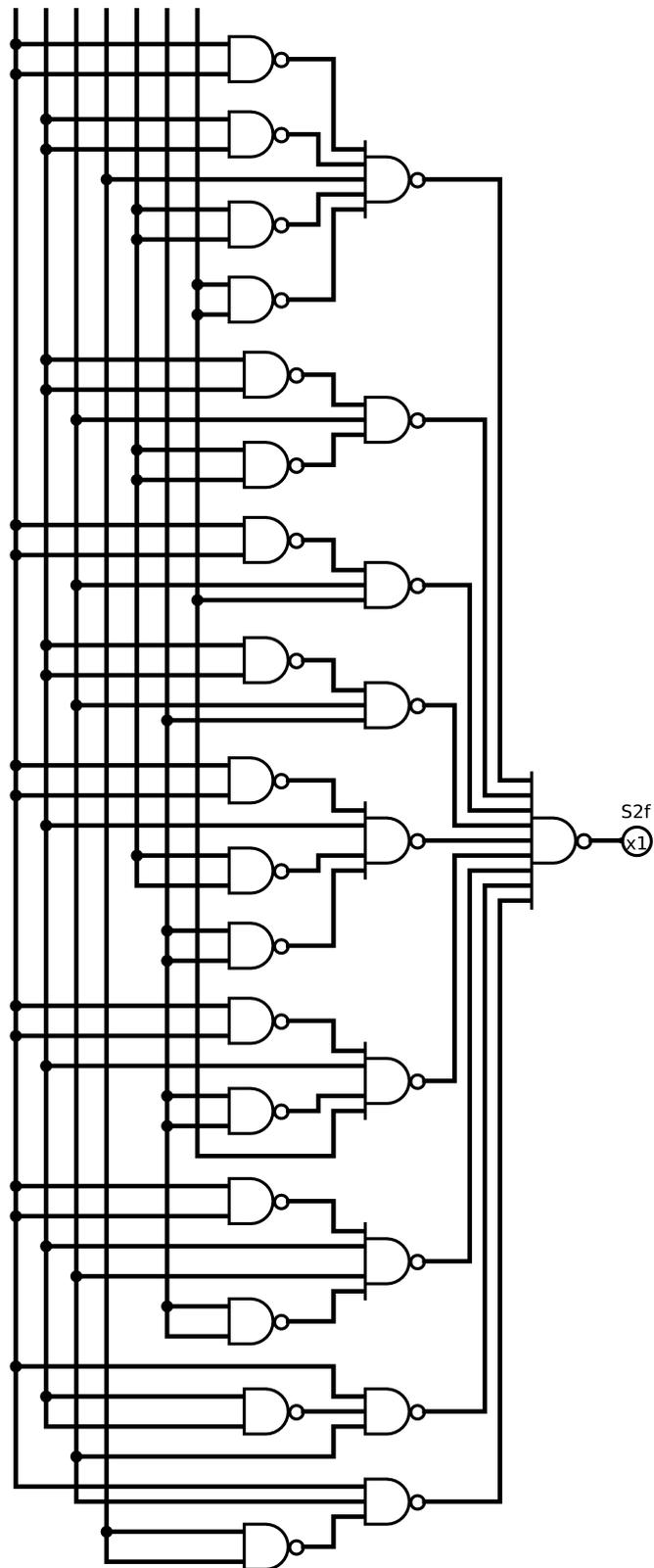
Figure 4.5: NAND gate realization of the input logic, continued from 4.4. Starting from the truth table the program *Logisim* built minimal logical expressions and converted them into the depicted NAND gate logic.
