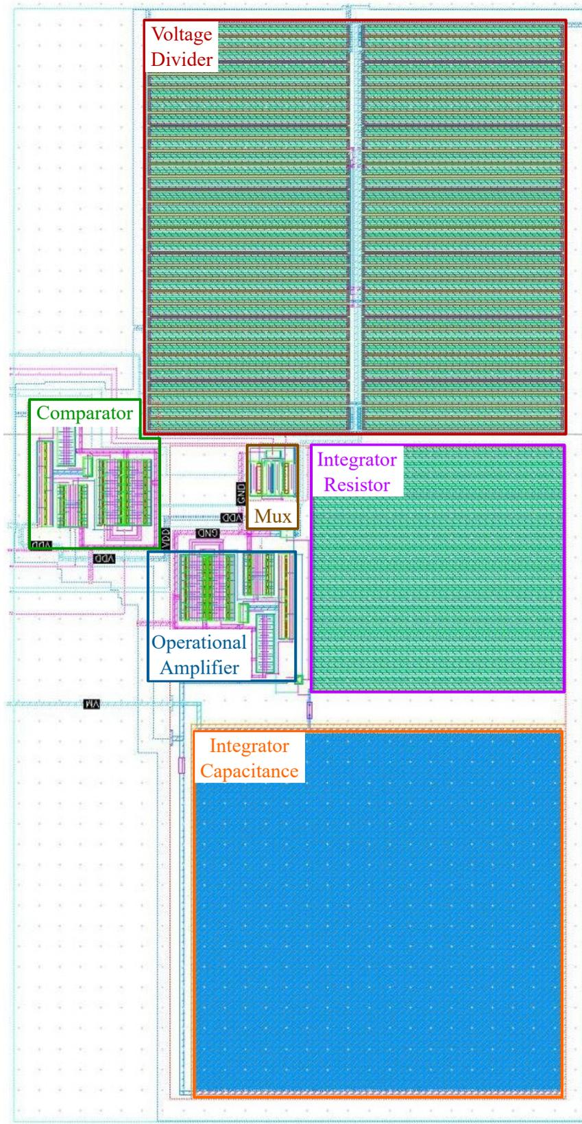
Figure 6.1: Layout of the Integrator with some peripheral components. The total area of these components amounts to  $0,035\ 108\ \text{mm}^2$  and is spun up by a rectangle measuring  $262\ \mu\text{m} \times 134\ \mu\text{m}$ .
