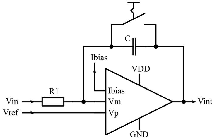
Figure 3.2: Model of an integrator resetting approach realized with a momentary switch. The bias current  $I_{bias}$  is needed inside the operational amplifier as a source to drive internal current mirrors which aim at reductions of the overall current consumption of the operational amplifier.
