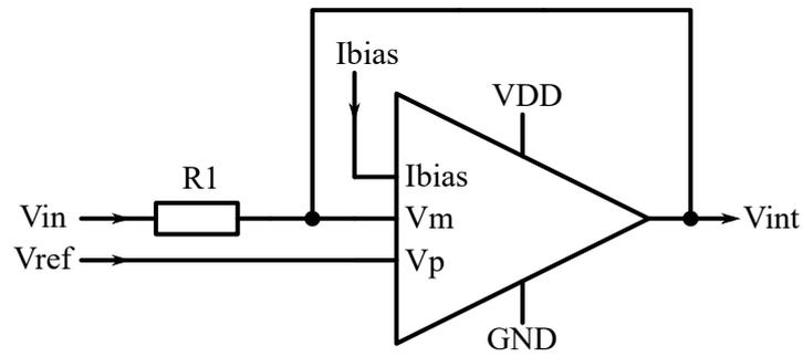
Figure 3.5: Result of Figure 3.2 when the switch is closed, an impedance converter, hence,  $V_{int}$  follows  $V_{in}$ .
