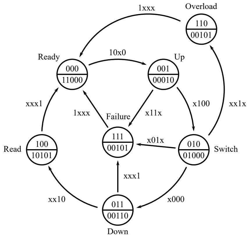
Figure 4.2: Depiction of the designed finite state diagram for managing the various states of the ADC. Based on this diagram truth Tables 1 and 2 are derived to be able to further derive the NAND gate logics presented in Figures 4.4, 4.5 and 4.6.
