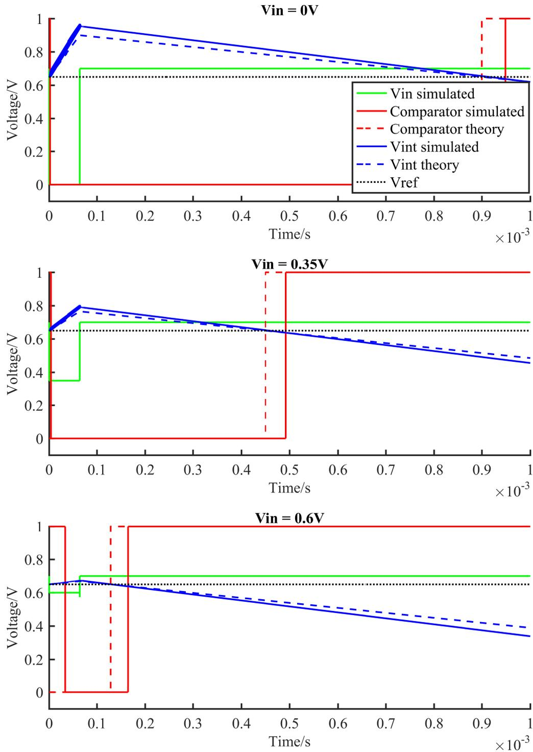
Figure 5.2: Comparison of theoretically calculated and simulated loading and unloading behaviors of the ADC for different constant input voltages  $V_m$ .
