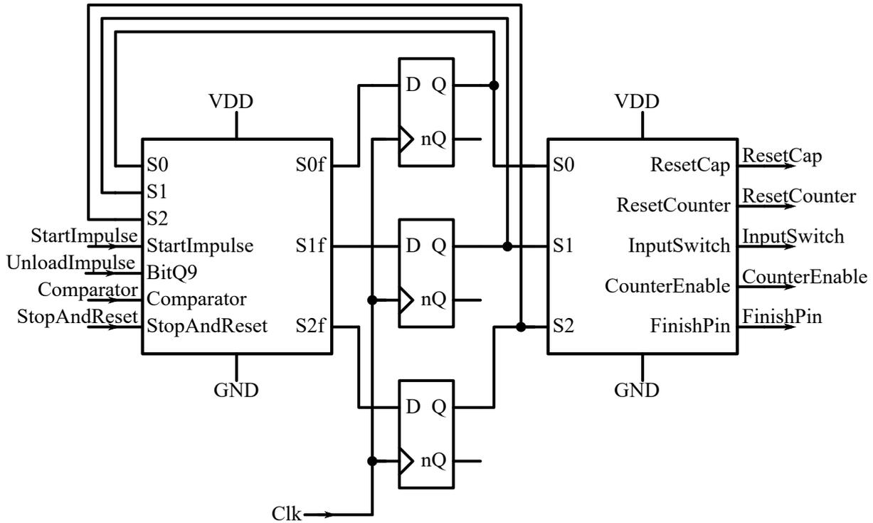
Figure 4.3: State machine split up into an internal logic, a unit for state persistence (D-flipflop array, one flipflop for each of the state bits  $S0$ ,  $S1$ ,  $S2$ ), and an output logic component (shown in order from left to right). Input and output stages are realized as NAND gate logic and shown in Figures 4.4, 4.5 and 4.6.
