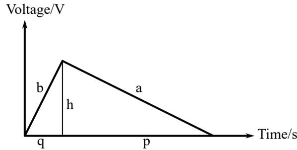
Figure 3.6: Model of the loading and unloading behavior of a dual slope analog digital converter. The slopes of  $b$  and  $a$  are indirectly proportional to the associated times  $q$  and  $p$ .
