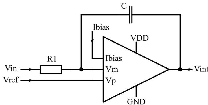
Figure 3.4: Result of Figure 3.2 when the switch is open, the integrator.
