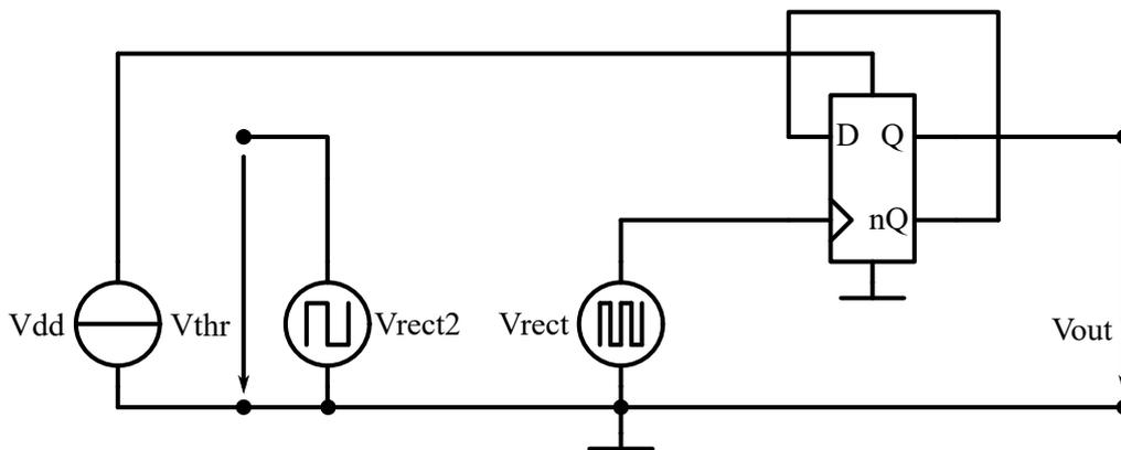
Figure 5.3: Testbench for optimizing the D-flipflop component presented in Figure 4.9. The optimization aims for two goals, the minimization of current consumption as well as for the correctness of the output signal. Thus, an ideal output signal form  $V_{thr}$  is artificially generated by  $V_{rect2}$ .
