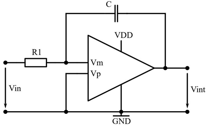
Figure 3.1: Integrator model based on an opamp operated in negative feedback loop. The capacitance causes the derivation of the feedback voltage. Hence, the opamp compares a signal with it's derivation and tries to eliminate the difference of the incoming signals. This results in integrating behavior.
