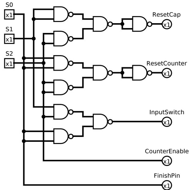
Figure 4.6: NAND gate realization of the output logic. Starting from the truth table the program *Logisim* built minimal logical expressions and converted them into the depicted NAND gate logic.
