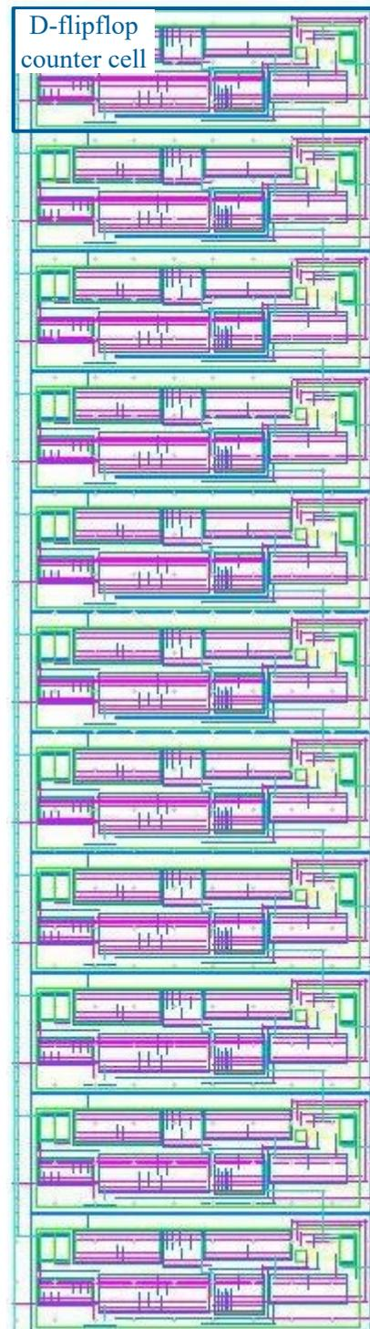
Figure 6.2: Layout of the counter sketched in 4.8. Single counter cells are designed to have an oblong outline shape to be able to be stacked adaptable. The total area of the counter component amounts to  $0,011492 \text{ mm}^2$  and is spun up by a rectangle measuring  $68 \mu\text{m} \times 169 \mu\text{m}$ .
