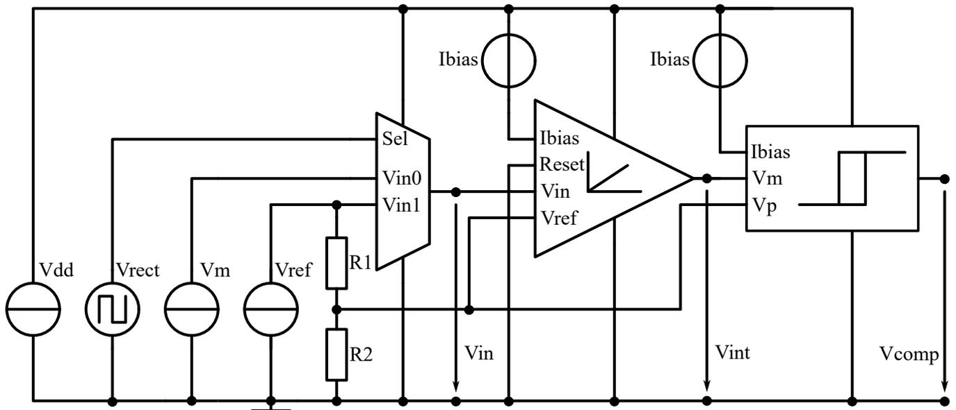
Figure 5.1: Testbench for current consumption and validation tests of the ADC's core components. A voltage  $V_m$  imitating the input signal's voltage level to convert is applied to compare with the theoretically evaluated behavior.
