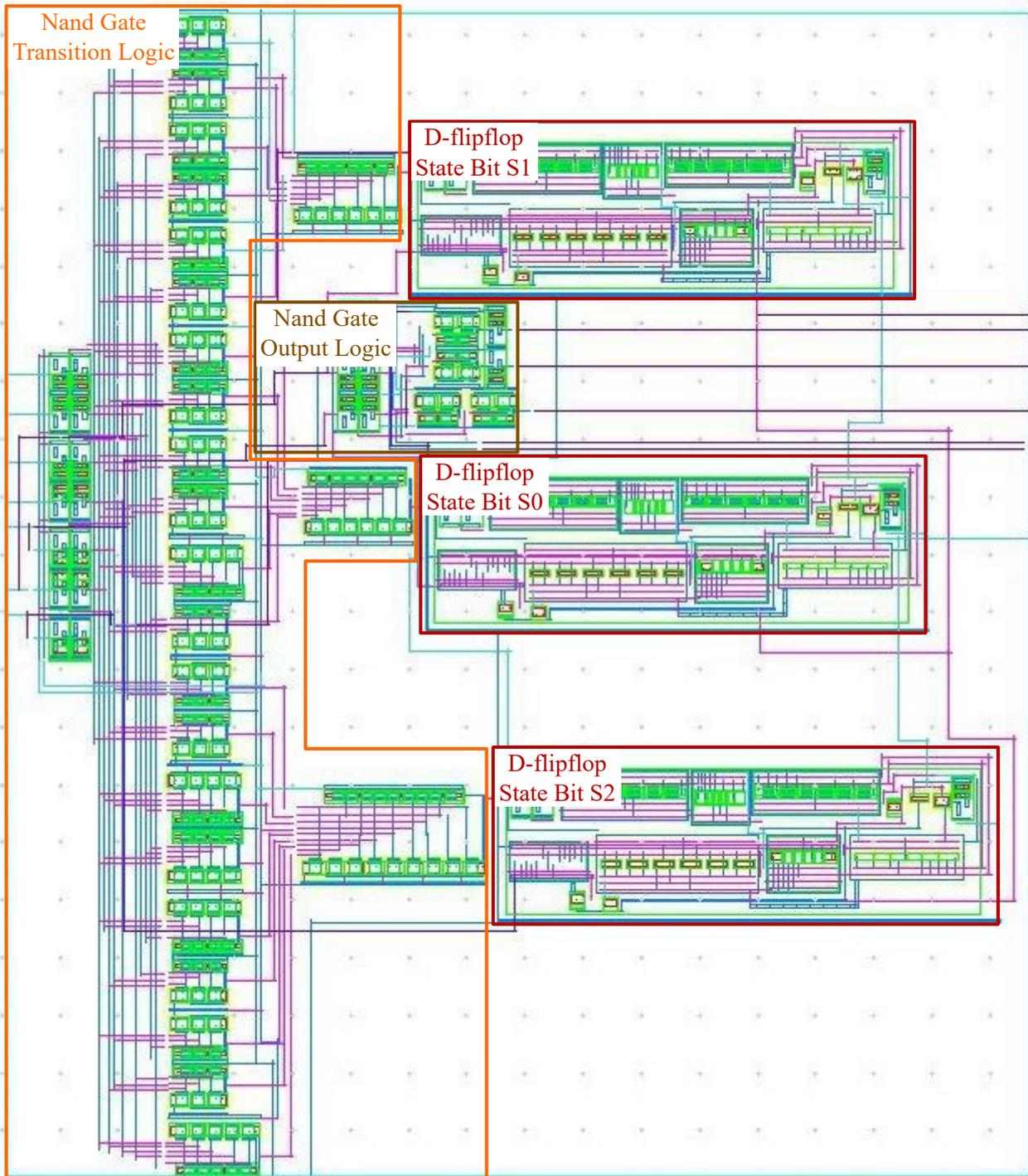
Figure 6.3: Layout of the state machine from Figure 4.3. The total area of the entire state machine component amounts to  $0,010\,706\text{mm}^2$  and is spun up by a rectangle measuring  $106\mu\text{m} \times 101\mu\text{m}$ .
