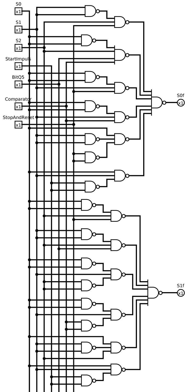
Figure 4.4: NAND gate realization of the input logic. To be continued by 4.5
