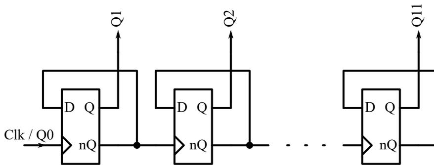
Figure 4.8: Assembly used for the realization of the 11 Bit counter. Due to the asynchronous design peak currents are reduced compared to a synchronous counter. The jitter induced by this design should have very little impact because of the relatively low operation frequency.
